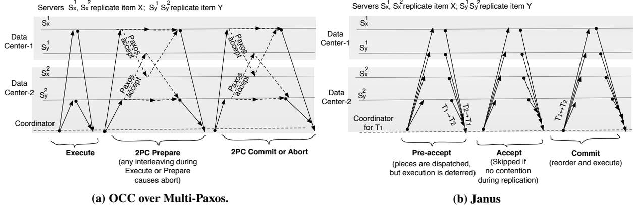
Figure 1: Workflows for committing a transaction that increments  $x$  and  $y$  that are stored on different shards. The execute and 2PC-prepare messages in OCC over Multi-Paxos can be combined for stored procedures.
