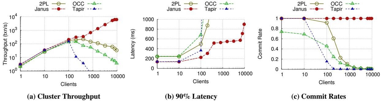
Figure 6: Performance in the geo-replicated setting for the TPC-C benchmark with increasing load and contention as controlled by the number of clients per partition.
